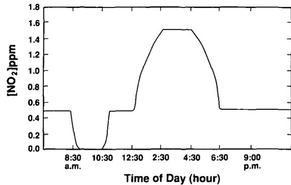
FIG. 1. Schematic showing the timing and concentration of the daily  $\text{NO}_2$  profile.
