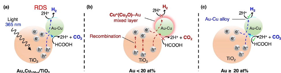
Figure 9. Schematic illustration of the proposed mechanism for the H 2 evolution from formic acid dehydrogenation by Au–Cu/TiO 2 photocatalysts.
