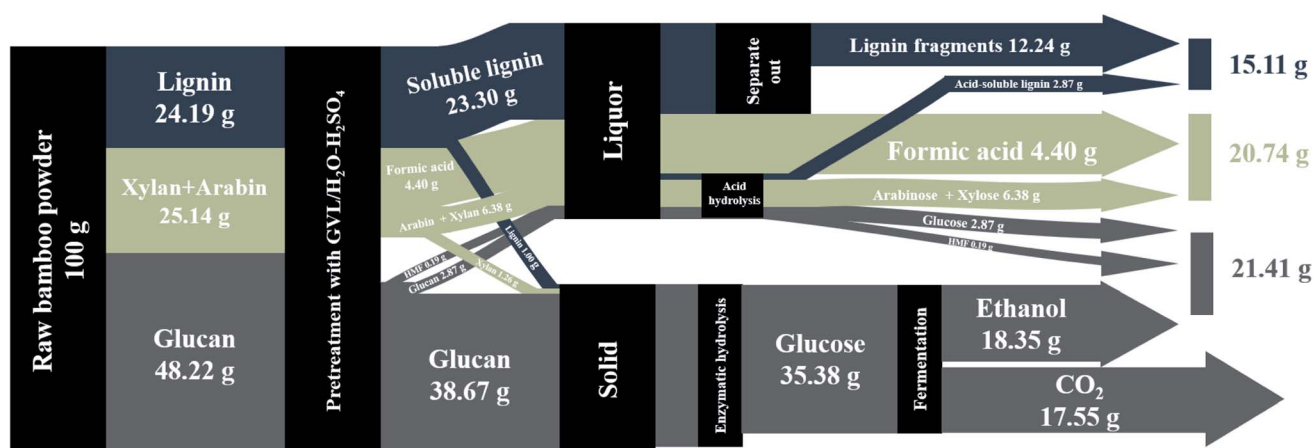
Fig. 8 Mass balances of bamboo substrates of ethanol production by GVL/H 2 O pretreatment (at 140 °C for 120 min with GVL : H 2 O = 8 : 2 and 75 mmol L -1 H 2 SO 4 ).
