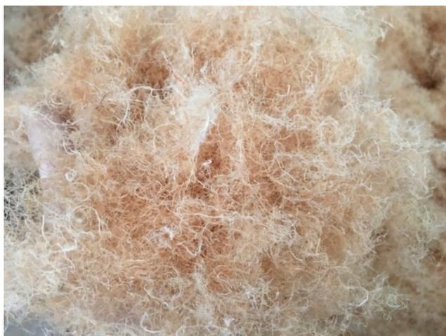
Figure 1. As-received raw bamboo fibers.
