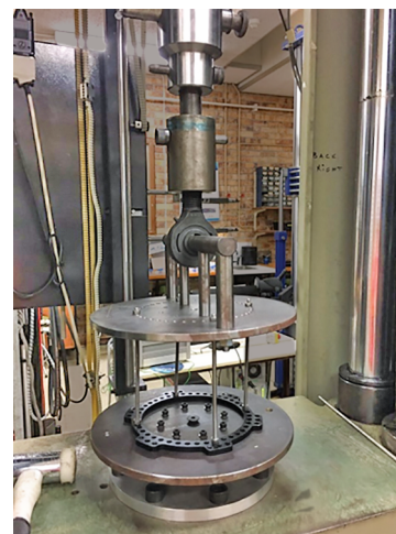
Fig. 2: A four-rod test sample mounted in the custom jig before testing in the Zwick 1484 Universal Testing Machine
