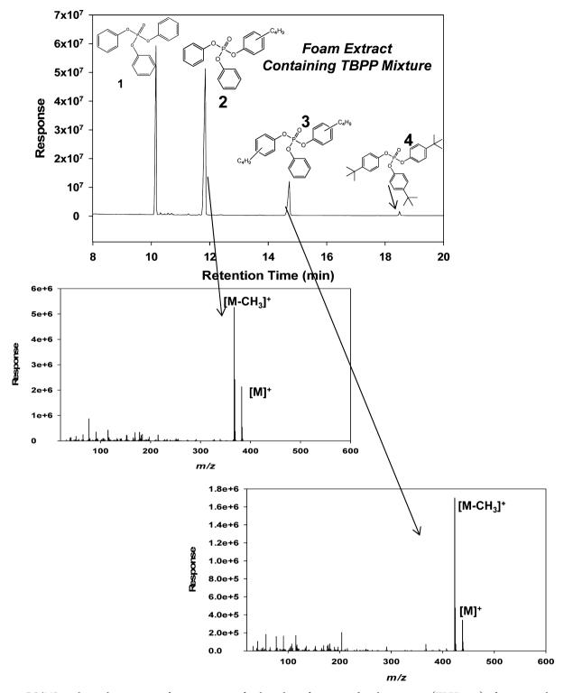
**Figure 1.** GC/MS total ion chromatogram from an extract of polyurethane foam treated with a mixture (TBPP mix) of aromatic phosphates including triphenyl phosphate (TPP) (1), 4-(tert-butyl)phenyl diphenyl phosphate (2), bis(4-(tert-butyl)phenyl) phenyl phosphate (3), and tris(4-(tert-butyl)phenyl phosphate (TBPP) (4). Structures 2 and 3 are hypothesized based on high resolution mass spectrometry analysis and the confirmation of structure 4.
