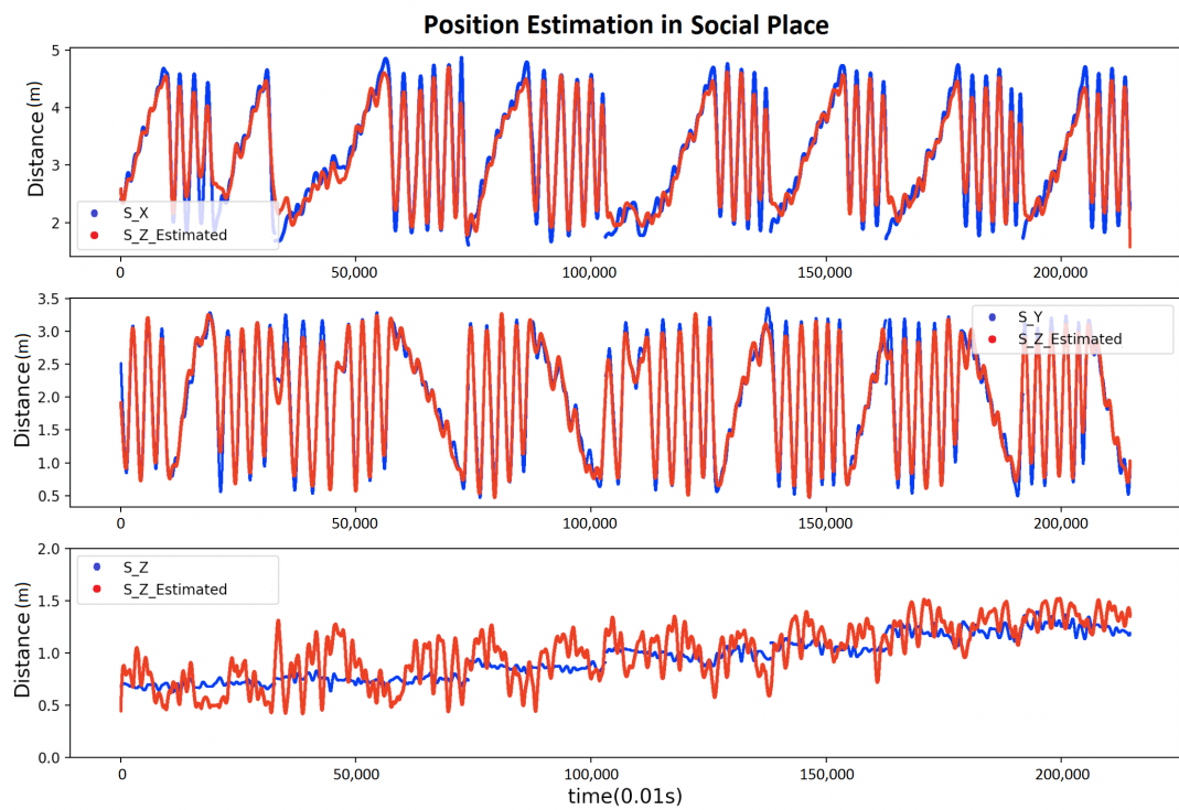
Figure A3. Comparison of the true coordinate with the estimated coordinate (social place experiment).
