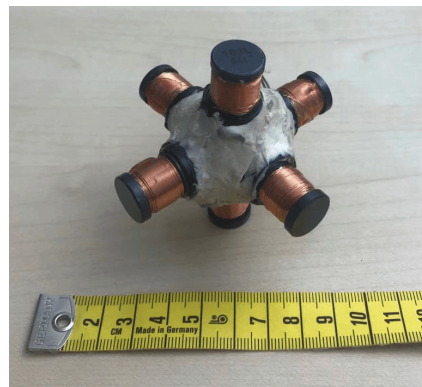
Figure 5. Receiver coil ( 8.5 \times 8.5 \times 8.5 cm and 6.6 mH in inductance of each axis).
