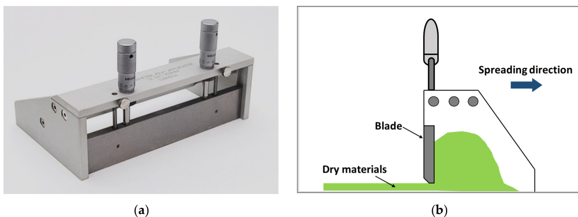
Figure 6. Micrometer applicator for preliminary jetting test. (a) Micrometer applicator. (b) Preliminary jetting test.
