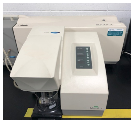
Figure 3. Equipment of particle size distribution (Hydro 2000MU) (Malvern, Worcestershire, UK).
