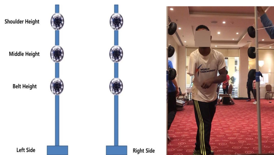
Figure 2. Front view of ROXs Pro sensors set up individually for each athlete's height; left (schematic), right (data collection).
