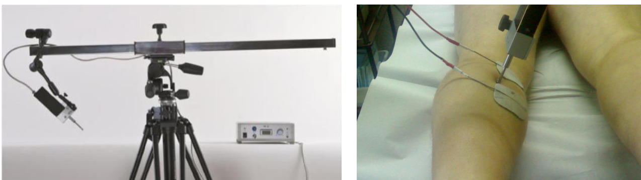
Figure 3. A TMG apparatus with a linear displacement sensor (left) was used to detect contractile properties while two self-adhesive electrodes were positioned distal and proximal to the thickest part of the muscle belly (right).
