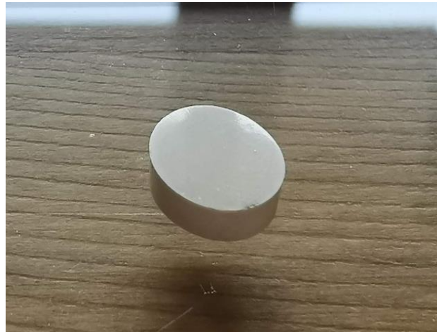
Figure 1. Biodentine sample (8 × 3 mm) removed from the PVC form.
