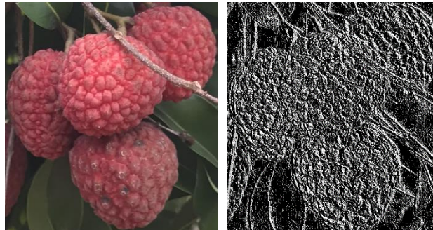
Figure 10. Local binary pattern (LBP) operator representation of a lychee image.
