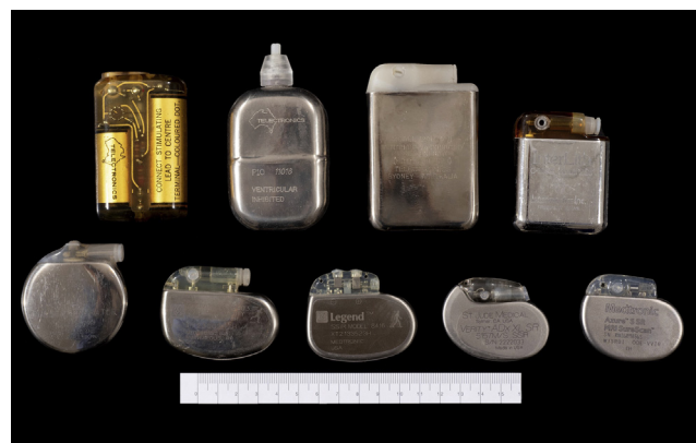
Figure 2 Examples of the pacemakers the patient received. From left to right, top to bottom: Teletronics P6 (1969), Teletronics P10 (1972 & 1974), Teletronics 120B (1976), Intermedics 223-01 (1980), Medtronic Mirel VL (1980), Medtronic Activatrax VVI+ (1986), Medtronic Legend 8416 (1995), St Jude Verity ADX 5156 (2008), Medtronic Azure SR (2021).
