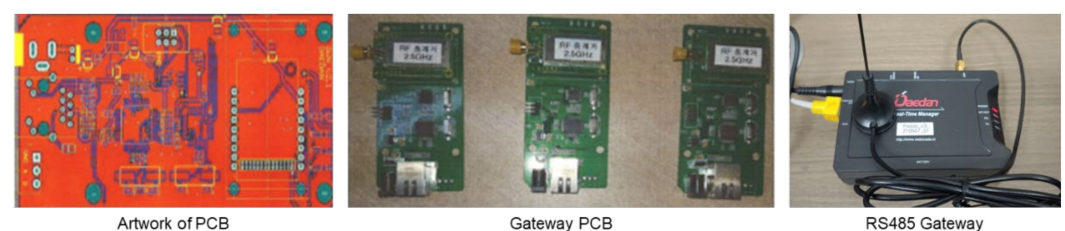
Figure 4. RS485 gateway for CPMS.
