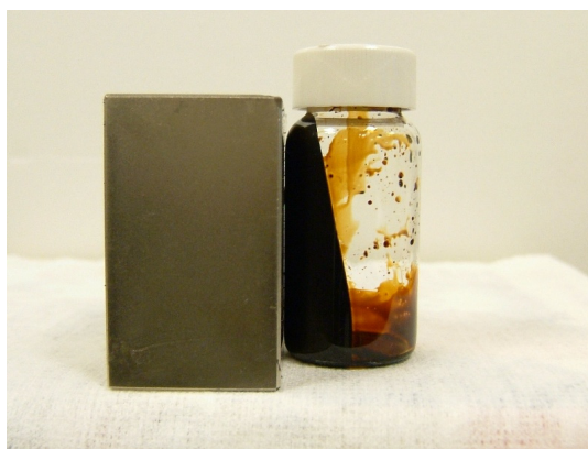
Figure 4. The magnetic effect on the ferrofluid.
