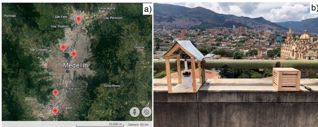
Fig. 1. a) Location of test sites in Valle de Aburrá, Colombia (Google earth) b) Sulfates and chlorides candles installed at S1.
