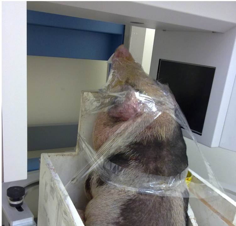
Figure 2 Experimental setup. The experimental setup for the CBCT scan of a typical subject. The pig was restrained on a purpose-built workbench using transparent tape, and the mandible was positioned within the center of the region of interest with the guidance of an optical localizer in the shape of a cross.
