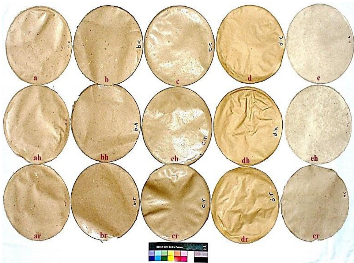
Figure 2. Paper sheets produced from wood species and after heating and iron rusting treatments; Schinus terebinthifolius (a), Erythrina humeana (b), Tectona grandis (c), Pinus rigida (d) and Juglans nigra (e). h, heated; r, iron-rusted.
