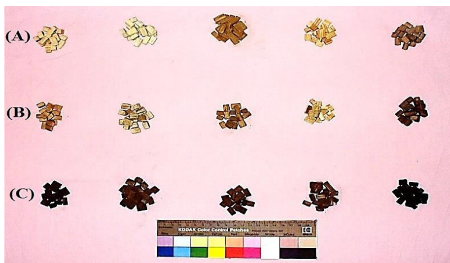
Figure 1. Groups of five age-accelerated wood species: (A) control, (B) heated and (C) rusted.
