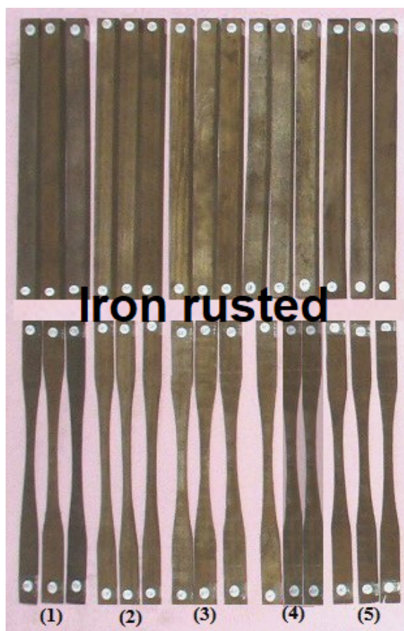
Figure 3. Wood samples with different treatments (heated and rusted woods) compared to control treatment (untreated wood) prepared for the testing of their mechanical properties. (1) Schinus terebinthifolius , (2) Pinus rigida , (3) Tectona grandis , (4) Erythrina humeana and (5) Juglans nigra .
