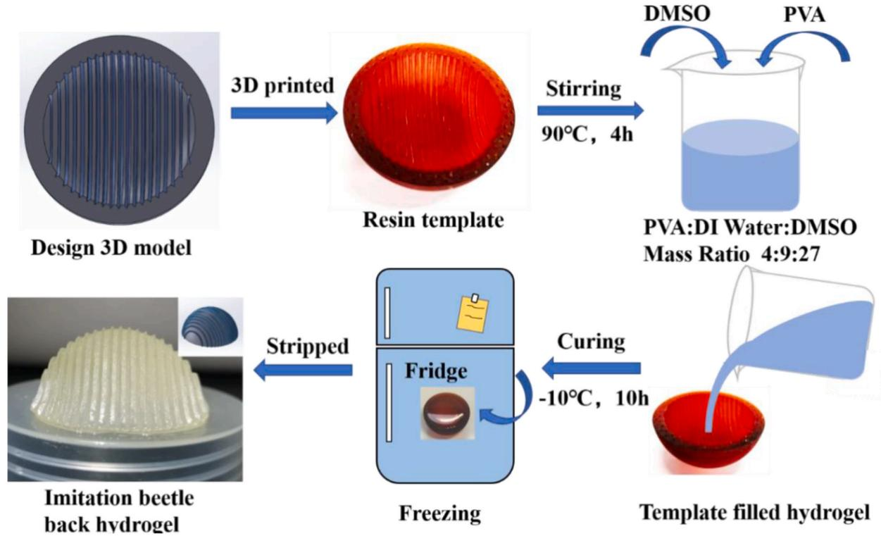
Figure 2. Schematic diagram of the preparation process of hydrogel-like beetle back structure.
