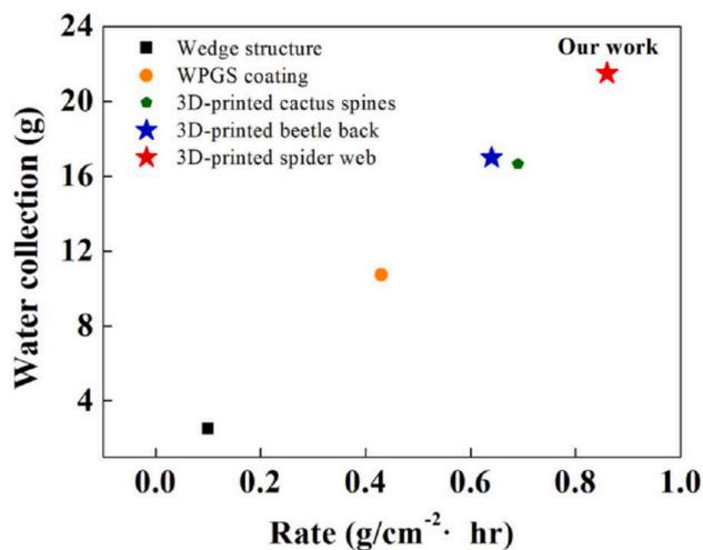
**Figure 6.** Comparison of the water collection effect between our work and previously reported works by other processing methods.
