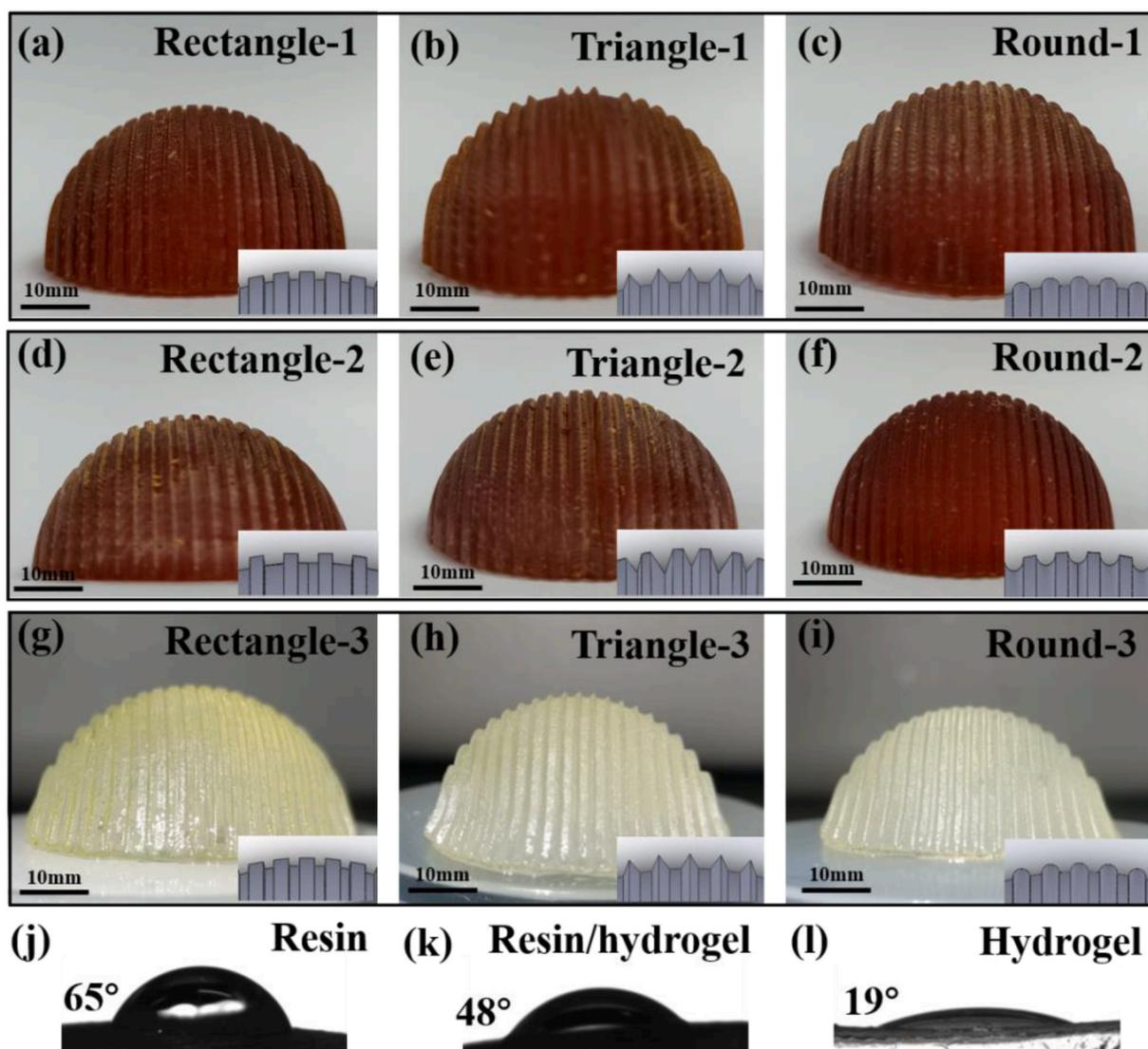
**Figure 3.** 3D printed beetle back model. (A–C) 3D printed beetle backs with different structures on convex surfaces; (D–F) 3D printed beetle backs with different structures on concave surfaces; (G–I) Hydrogel beetle backs with different structures; (J–L) Contact angles of the printed resin material, resin coated hydrogel and PVA hydrogel material surfaces. The inset corresponds to a partial enlargement of the beetle back model.
