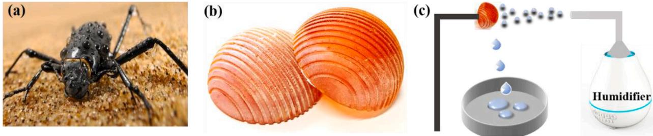
**Figure 1.** Inspired by the Namib beetle and biomimetic preparation of the beetle's back. (A) Natural beetle using its back to collect water [13]. (B) Physical view of the 3D printed beetle back. (C) Schematic diagram of the printed beetle back simulating a water collection device in a high humidity environment.
