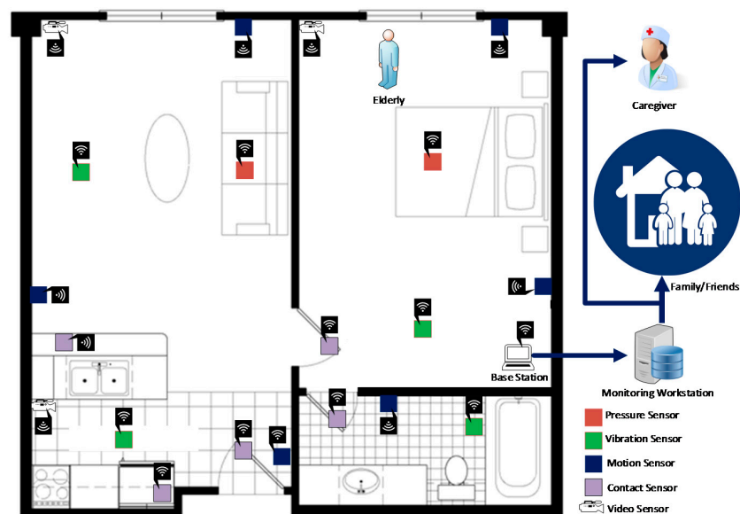
Figure 4. Sample schematic setup of a smart apartment for elderly care based on different ambient sensors.
