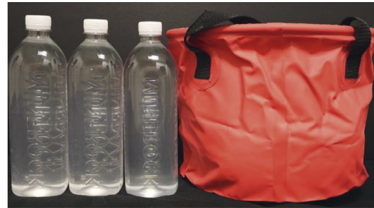
FIGURE 1: Fifty-fold concentrated SGW in 1 L bottles and a 20 L-sized bucket provided to the participants for dilution.
