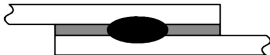
Figure 4. Weld-bonded joints result from the combination of adhesive bonding with resistance spot-welding based on [23].
