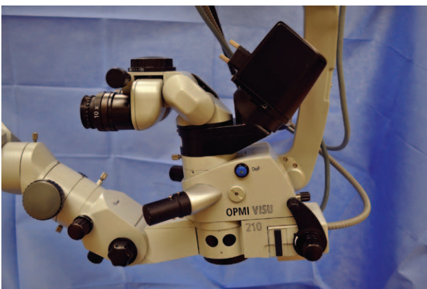
Fig. 1. TrueVision image capture module (black box-shaped apparatus) attached to oculars of standard surgical microscope.
