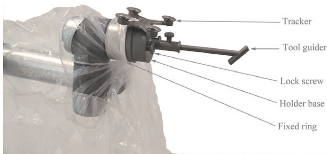
Fig. 3 TianJi Robot navigation and positioning tools installation, including fixed ring, tracker, tool guider, lock screw, and holder base.
