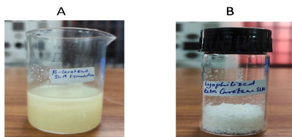
Fig. 4. Visual appearance of (A) solid lipid nanodispersion of optimized formulations and (B) lyophilized powder.
