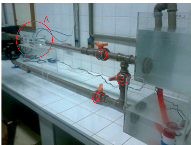
Fig. 1 - Steady flow hydrodynamic workbench photo Highlighted: A (test chamber), 1 (top spherical valve), 2 (bottom spherical valve) and 3 (maintenance spherical valve)
