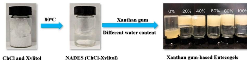
Figure 1. The preparation process of xanthan gum-based eutectogel.
