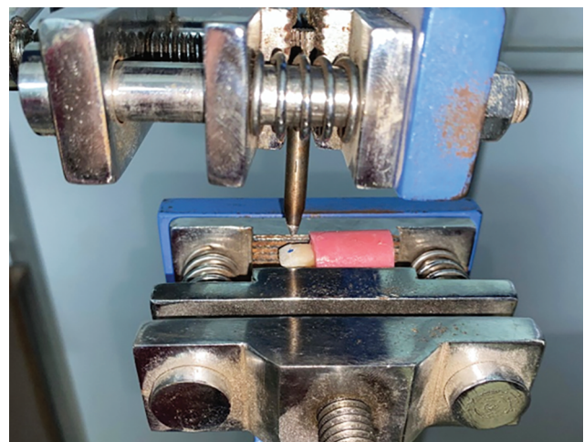
Fig. 7: Sample loaded under universal testing machine
