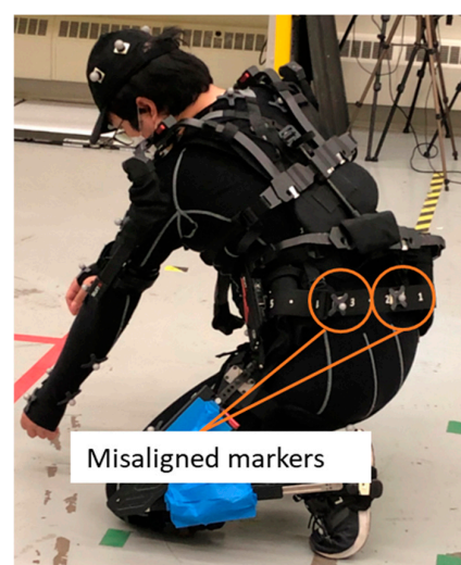
Figure 18. The markers on the exoskeleton misaligned with the human body.
