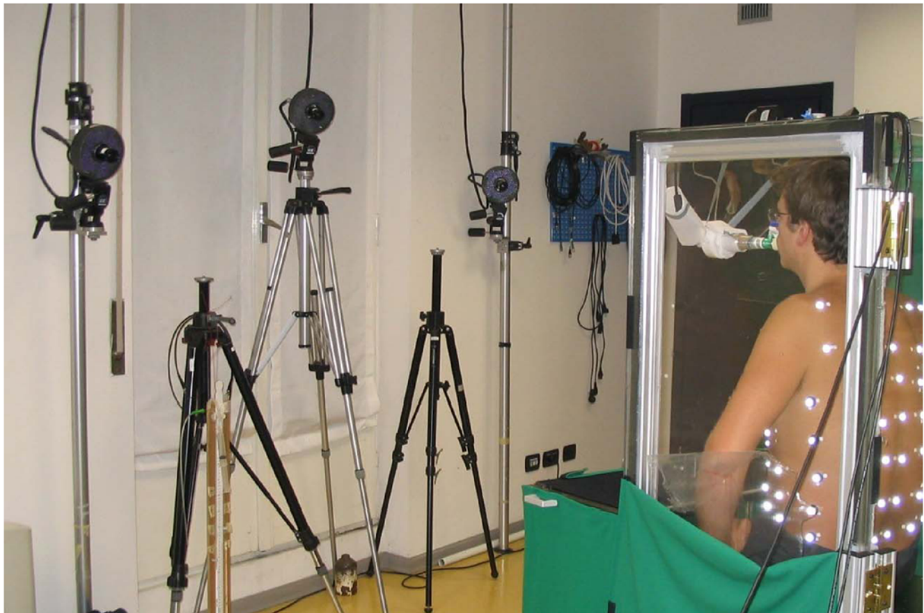
Figure 8. Photograph of a subject inside the transparent whole body plethysmograph with body surface markers for optoelectronic plethysmography in place. The cameras recording motion of the anterior markers are shown in the background. doi:10.1371/journal.pone.0005550.g008
