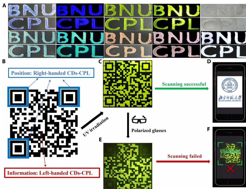
Fig. 5. CDs-CPL for printing circular polarization luminous patterns and implementing multilevel anticounterfeiting. (A) Dispensing printed CPL and BNU circularly polarized luminous patterns on flexible PET fabric using full-color CDs-CPL. (B) Custom QR code creation. (C and D) First-level anticounterfeiting process of CDs-CPL based on PL characteristics. (E and F) Secondary anticounterfeiting process of CDs-CPL based on CPL characteristics.
