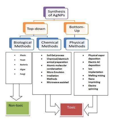
Figure 2. Different method used for the synthesis of (AgNPs) nanoparticles.
