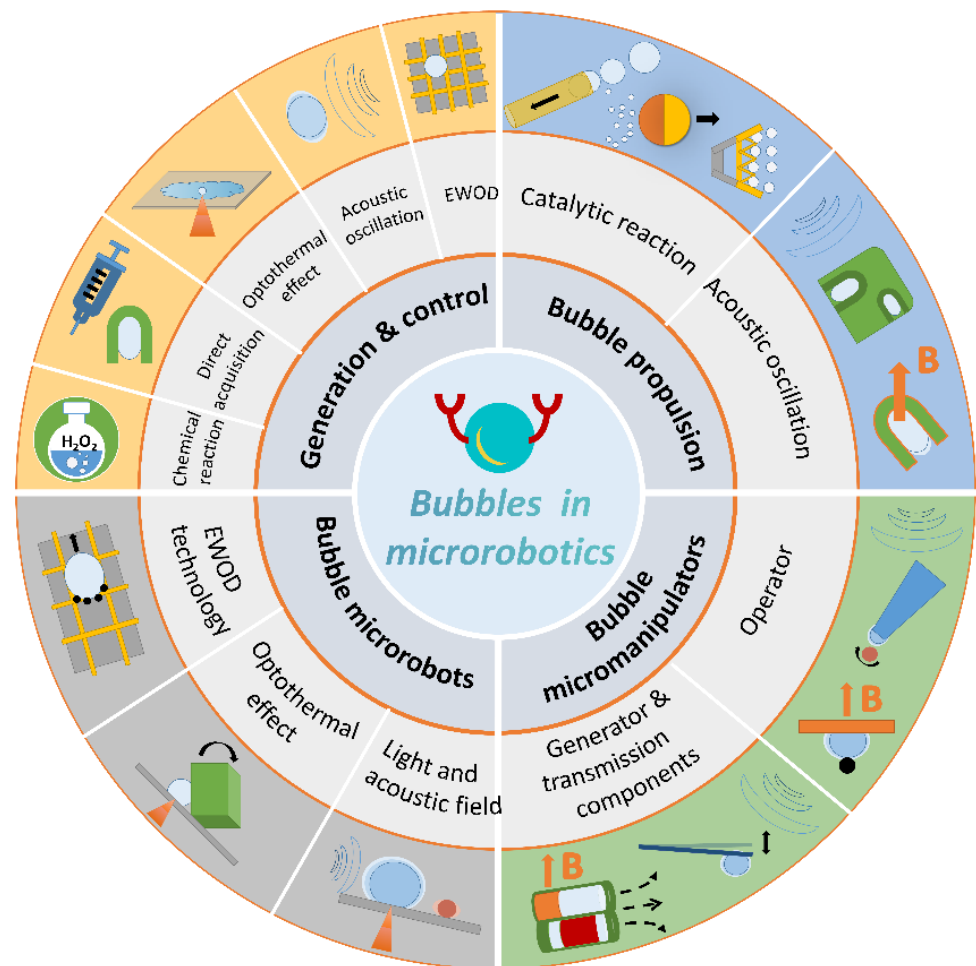
Figure 1. The generation and control methods of the bubbles and their roles in microrobotics.
