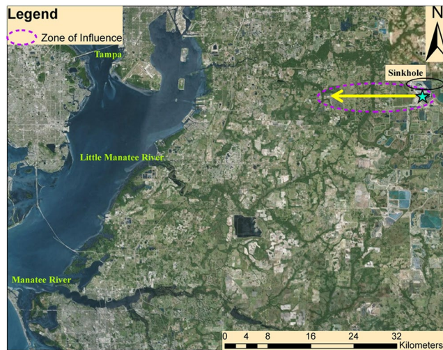
Figure 1. Location of the sinkhole as depicted by the blue star, and the general direction of groundwater flow shown by the yellow arrow. The area circled in black represent approximate well locations. The dashed area in purple is a conceptual representation of the zone of influence of the plume after 20 years, based on advection, diffusion, and adsorption. The zone of influence would be smaller if any wells in the region are active. (Figure created using ESRI ArcGIS 10.0 software, https://www.esri.com/en-us/arcgis/about-arcgis/overview . World Imagery basemap is included in ArcGIS 10.0 and is attributed to ESRI, DigitalGlobe, GeoEye, Earthstar Geographics, CNES/Airbus DS, USDA, USGS, AEX, Getmapping, Aerogrid, IGN, IGP, swisstopo, and the GIS User Community).
