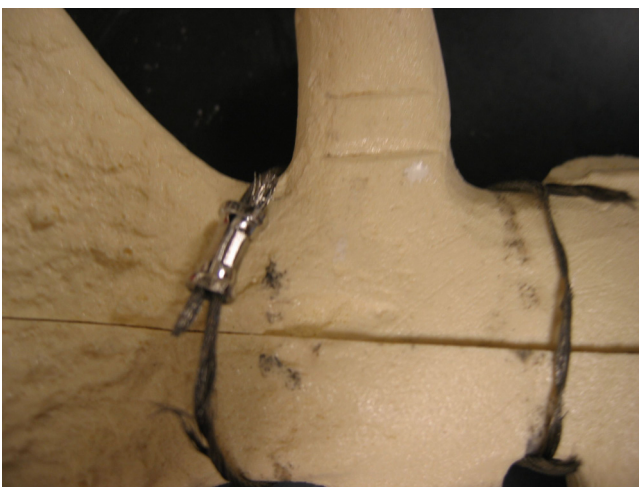
Figure 6 Site of failure in one model fixed with the figure-of-eight stainless steel cable that exhibited catastrophic failure during testing.
