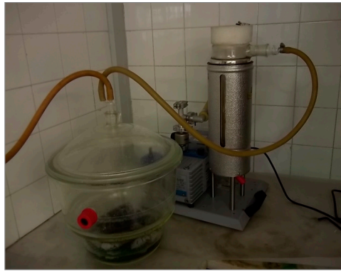
Figure 3. Porosity test equipment.
