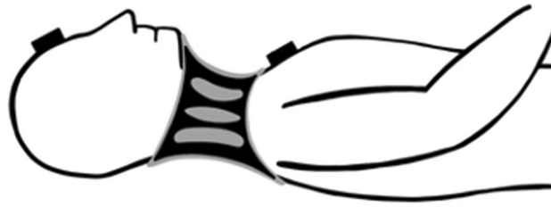
Figure 2. A fresh human cadaver is positioned supine on a spine board with a cervical collar; the motion trackers are fixed to the forehead and to the sternum.
