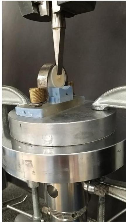
**Figure 2.** Micro-shear bond strength evaluation with INSTRON.
