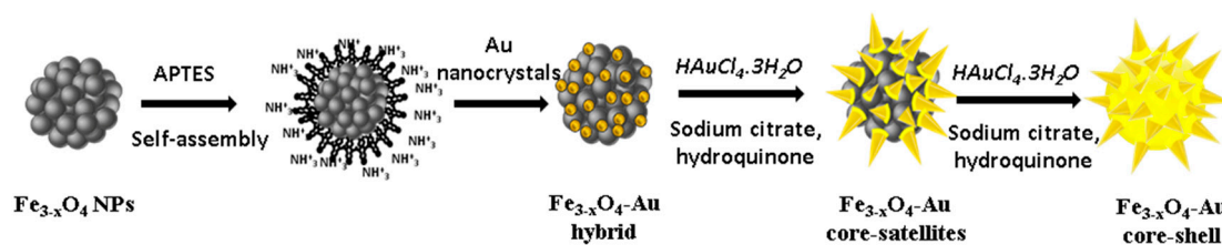
Figure 1. A schematic description of the different experimental steps involved in the production of star-shaped, \text{Fe}_{3-x}\text{O}_4 -Au core-shell particles.
