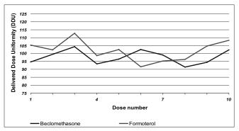
Fig. 2: Delivered dose uniformity of the formulation using a 0.48 mm actuator
