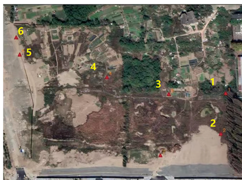
Figure 11. Venue location layout. We found these 6 points in the abandoned oil storage area, numbered 1–6, and marked them on the satellite map, and then took 3 soil samples at different depths from each point (Map data ©2022 Google).
