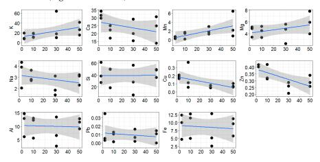
**Figure 2.** Changing trend of element content in dust collected from the leaf surface (g kg<sup>-1</sup>) in line distance to the road (2–50 m), drawn with smoothing lines (95% confidence interval).
