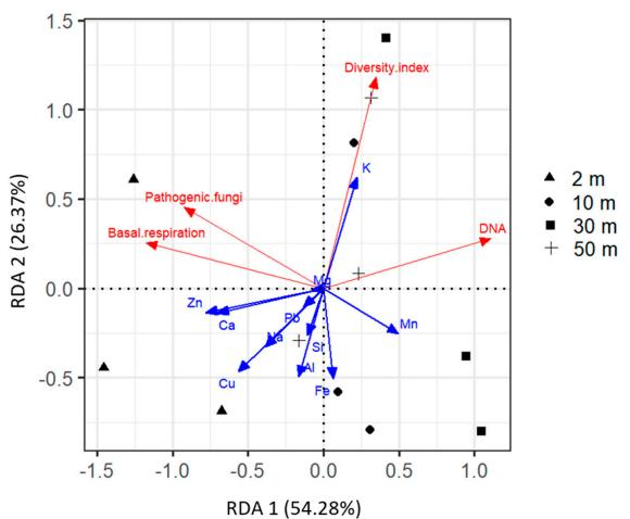
**Figure 10.** RDA ordination triplot showing the relationships of microbial properties (red arrows) and chemical elements (blue arrows) of the dust from leaves' surface at different distances from the road (2–50 m).
