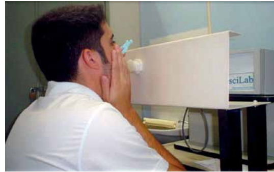
Figure 2. Example of forced oscillation respiratory impedance measurement
