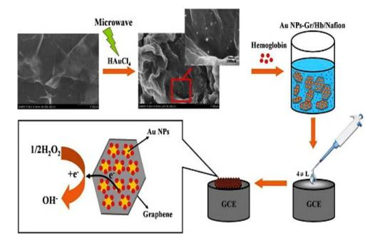
**Figure 9.** Fabrication steps of AuNPs–Graphene/Hb/Nafion/GC electrode and electrocatalytic activity for H<sub>2</sub>O<sub>2</sub>. Adapted from [87], with permission from ©2014 Elsevier.
