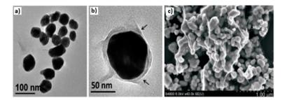
**Figure 7.** TEM images of the Au-encapsulated GO nanoparticles at (**a**) low magnification; (**b**) high magnification, adapted from [140], with permission from ©2013 Royal Society of Chemistry and (**c**) SEM image of GO-wrapped AuNPs, adapted from [141], with permission from ©2014, 2015 Wiley.
