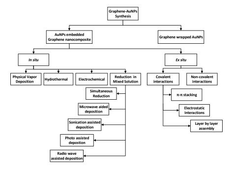
Figure 5. Schematic diagram of the graphene–AuNPs synthesis procedures.
