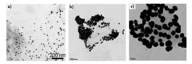
**Figure 4.** TEM image of GO–AuNPs composites (**a**) *in situ* growth, adapted from [81], with permission from ©2014 Nature Publishing Groupand (**b**) and (**c**) *ex situ* decoration of 20 nm and 40 nm AuNPs on GO sheets respectively, adapted from [82], with permission from ©2010 Royal Society of Chemistry.
