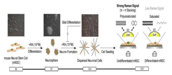
**Figure 14.** Schematic diagram representing the method to detect the undifferentiated and differentiated state of mNSCs using 3D GO-encapsulated AuNPs. Adapted from [139], with permission from ©2013 Elsevier.
