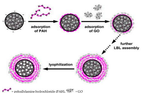
**Figure 8.** LBL fabrication process of Au@PLA–(PAH/GO)<sub>n</sub> microcapsule. Adapted from [148], with permission from @2013 Elsevier.
