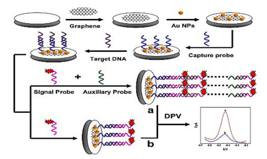
**Figure 10.** Schematic representation of the fabrication procedure of the DNA biosensor. (a) DPV cures from the super-sandwich biosensor; (b) DPV cures from the sandwich biosensor. Adapted from [167], with permission from ©2015 Elsevier.
