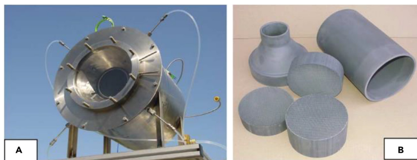
Figure 9. Design of honeycomb solar reactor
