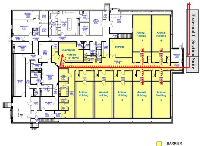
FIGURE 2 Floor plan of the SAF facility indicating cohort #2-6 founder population flow. The barrier is bordered with blue lines, and the location of the external C-section suite is shown. The flow of the piglets through the building is indicated, [continuous red line] from C-section in the external C-section suite to quarantine nursery and [interrupted red line] CDCD piglets from quarantine nursery to holding rooms
