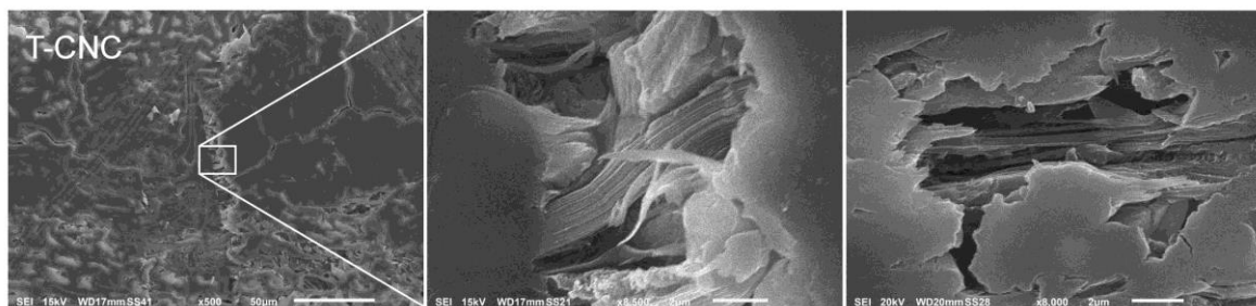
Figure 4. Creeps inside the glue-line of sample F (T-CNC) showing bundles of cellulose nanocrystals (center and right).
