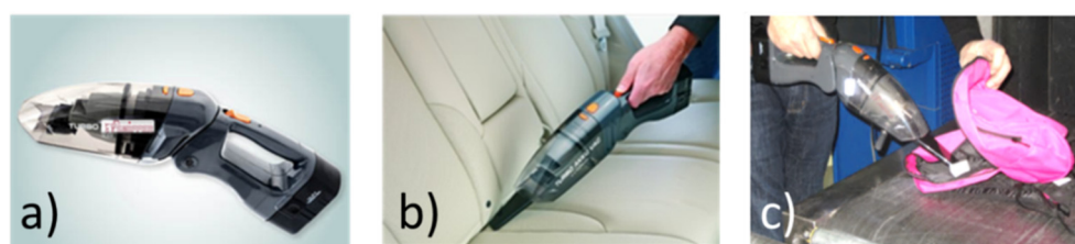
Figure 23. (a) ESP sampler system built into a commercial, battery-operated vacuum cleaner. Explosives particles and/or illicit drug residue were extracted from purposely contaminated environments (b,c) and placed onto cotton swabs inserted into the ESP sampler. Solid-vapor conversion and detection still needs to be performed by a separate stationary detector system.
