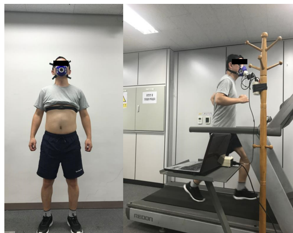
Figure 3. Example figures of the experimental equipment and process. During the experiment, participants wore a chest strap and a calorimeter to measure HR and EE, respectively. Each participant ran on a treadmill at a speed varying from 3 to 10 kph, which increased by 1 kph per every 2 min (total 16 min ran) and they were instructed to run at a constant speed as much as possible.
