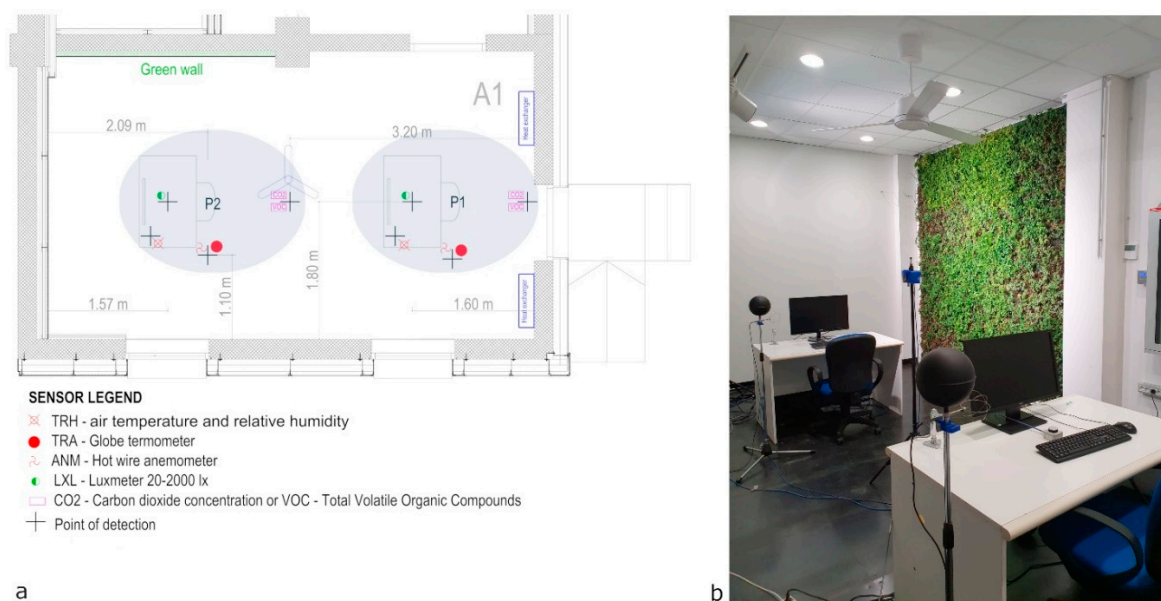
Figure 2. A1 room: (a) spatial distribution of sensors; (b) photo of the room set up.
